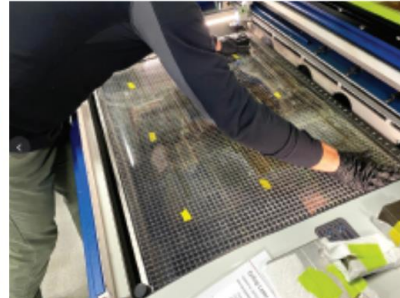
Mark centers of each shield on bed of cutter.
