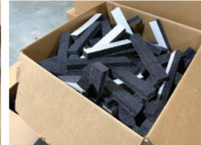
Cut foam to length and width using a shear, Xacto blade or scissors.
