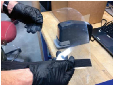
Line up elastic with edge of shield, slightly below the top of the plastic.
