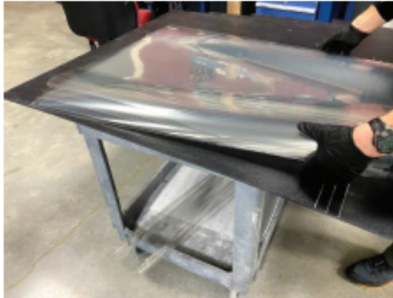
Cut clear plastic into rectangles that fit your laser cutter bed.
