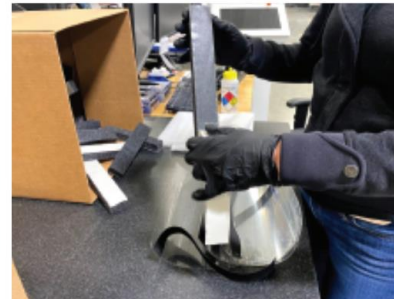
Remove liner from foam to expose the adhesive.
